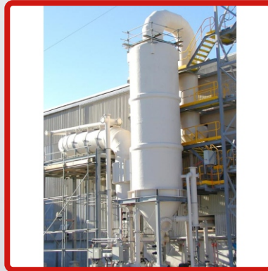
PP FRP WET PACKED SCRUBBER
